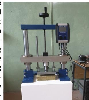
The dynamic stiffness of elastic insulation materials is an important material parameter in building acoustics and must be known, for example, to predict the resonance frequency of floating floors or double walls.
