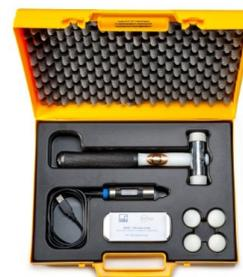
The new cross-hole analyzer (CHA) is designed for evaluation of concrete quality in deep foundations by the crosshole sonic logging method, it assesses concrete quality and consistency of drilled shafts and other cast-in-place concrete structures.
