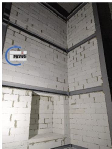
Figure 1 - Testing steel frame with prepared combustion chamber
